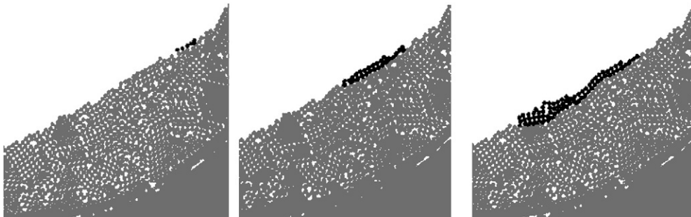
Figure 6. Sequence of pictures showing the development of an externally triggered avalanche (regime II). The rear front propagates downwards with a velocity equal to the depth averaged velocity \bar{v} of the avalanche. The velocity v_{\downarrow} of the head front is approximately equal to 2\bar{v} .
